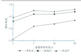
图 4 补加和调整溶剂后的硬度建立 Fig 4 Hardness development after solventmodification
