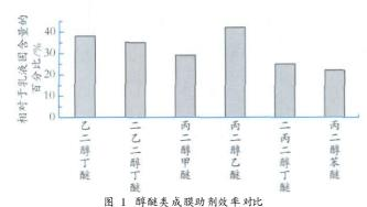
Fig 1 Performance comparison of film forming additive
